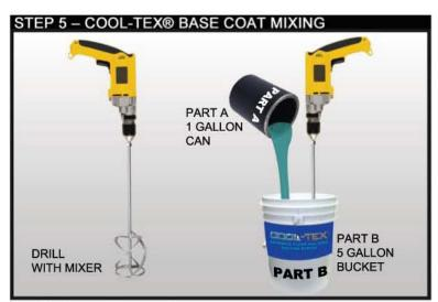
Mix COOL-TEX® Base Coat Part A and Part B components with mixing blade and drill prior to application. Begin by mixing Part B until smooth then slowly adding Part A, keeping a good vortex the entire time. Continue to mix for 2-3 minutes. Once mixed, material must be applied within 2 hours for best results. Material applied at the latter end of the open time will have a tendency to build and streak. Four gallon kit shown. Base coat is also available in one gallon kits.
