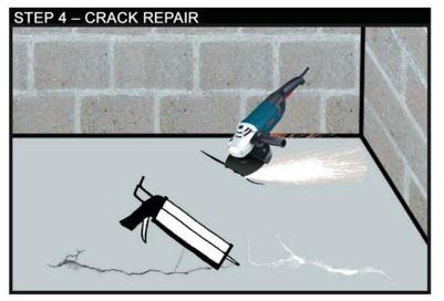
All cracks should be ground out, cleaned of any loose material, and filled with Roadware Concrete Mender in accordance with manufacturer's specifications\*. Once cracks are filled, the entire repaired area should be ground down to provide a smooth surface for application of COOL-TEX®. Concrete should be tested for excess moisture prior to application.
