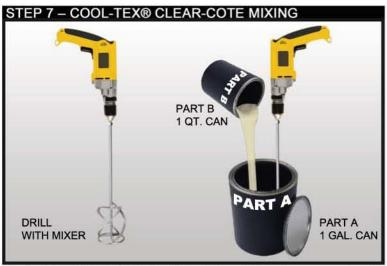
Mix COOL-TEX® CLEAR-COTE Part A and Part B components with mixing blade and drill prior to application. Begin by mixing Part A until smooth then slowly adding Part B, keeping a good vortex the entire time. Continue to mix for 2 – 3 minutes. Mixed material will have a milky appearance but will dry clear. Once mixed, material must be applied within 2 hours. Do not close the lid on unused material as pressure will build up in the can. COOL-TEX® CLEAR-COTE is available in 0.9 gallon kits.
